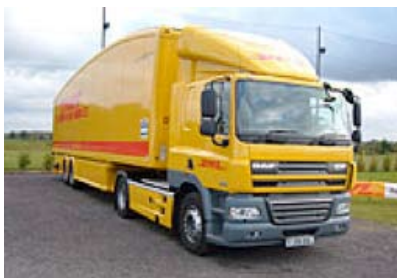
An example of an aerodynamic design – Deutsche Post DHL in the UK: The Teardrop Trailer
